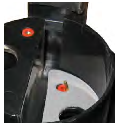
typical defect of an original spring pin
