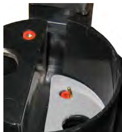
Typical defect of an original pin
